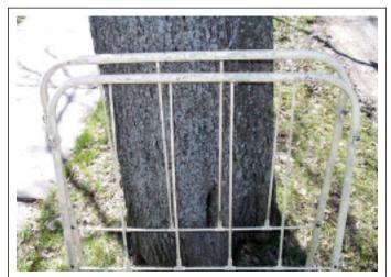
FIGURE 5.18 Baby's bed exhibiting deteriorated paint and evidence of teeth marks.
