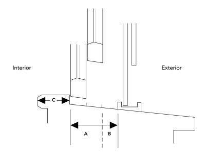
2. Sectional view of window (including storm window) showing window trough area, A and B, to be tested. Trough extends out to storm window frame. The interior window still (stool) is shown as area C. Interior window sills and window troughs should be sampled separately.
