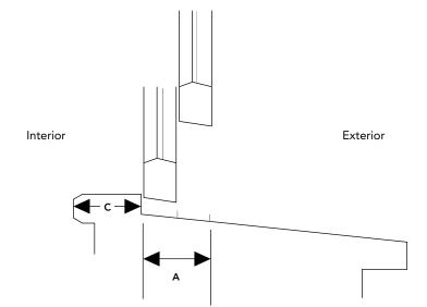
Sectional view of window (with no storm window) showing window trough area, A, to be tested. Trough is the surface where both window sashes can touch the sill when lowered. The interior window sill (Stool) is sown as area C. Interior window sills and window troughs should be sampled separately.
